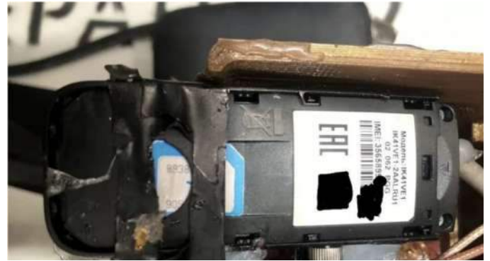
Figure 29. Modem and a SIM card of the Ukrainian mobile operator Kyivstar installed on the body of a Shahed UAV.
