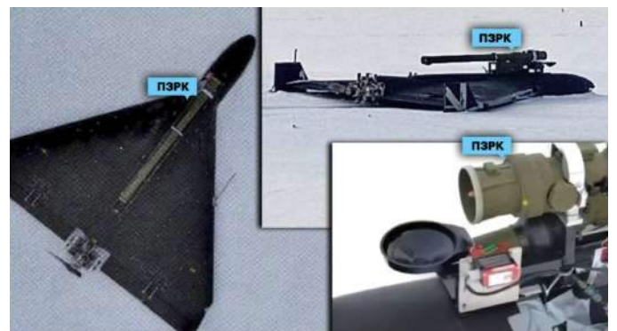
Figure 38. Serhii Beskrestnov (Flash). Russian Shahed UAV equipped with a MANPADS (Geran-4) 71 .
