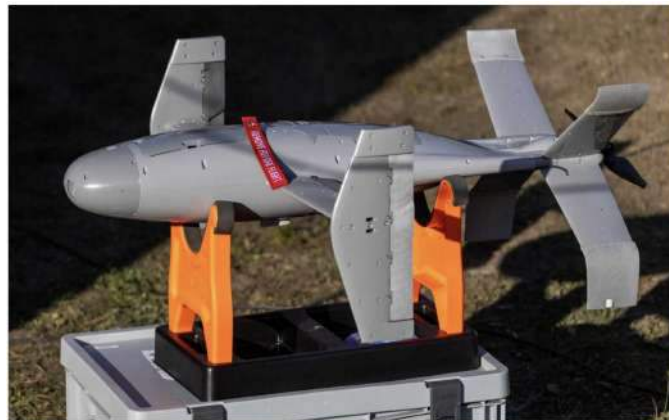
Figure 61. Militarnyi. Surveyor interceptor drone of the Merops anti-drone platform 134 .
