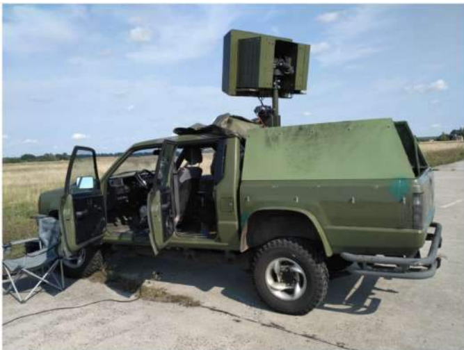
Figure 57. Militarnyi. Bukovel-AD electronic warfare system mounted on an off-road vehicle chassis. 2019 126 .
