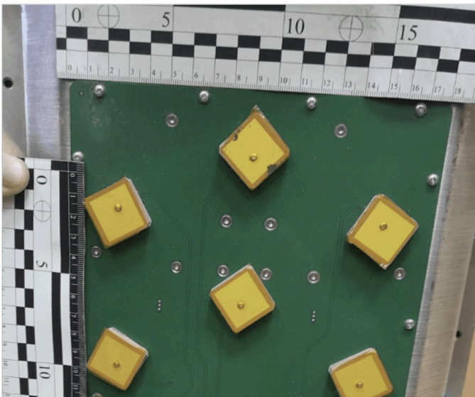
Part of the new Russian 16-element CRPA antenna Source: UNITED24 Media
